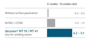
The analysis of various substrates using XPS (X-ray photoelectron spectrocopy) after passivation with deconex® MT 41 shows clear results: Our passivation method markedly improves the natural passivation layer. The ratio of chrome to iron or chromium oxide to iron oxide rises significantly. In the area of weld seams, the chrome and chromium oxide concentrations are also significantly increased with this process.
