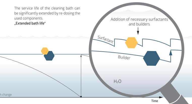
From an experience-based cleaning process to measurable process management ready for Industry 4.0
